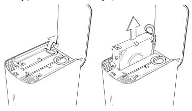
5. Gently slide the replacement drive assembly into the drive slot until is fully inserted.
